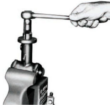
Figure 4 - Tightening the seat ring retainer (4)
