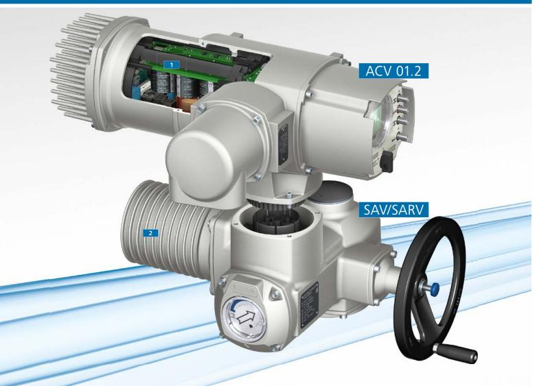
AUMA variable speed multi-turn actuators are the combination of SAV/SARV actuators and ACV 01.2 actuator controls. Variable speed is achieved by the integral frequency converter within the actuator controls. ACV 01.2 are based on the intelligent AC 01.2 actuator controls. Operation and integration of ACV into the DCS is comparable to AC.
