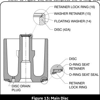
retainer. Remove the retainer lock ring with Truarc Pliers (BHGE Part No. 5153304).
