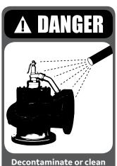
if necessary before pretesting or disassembly. Safety and environmental precautions must be taken for the decontamination or cleaning method used.
