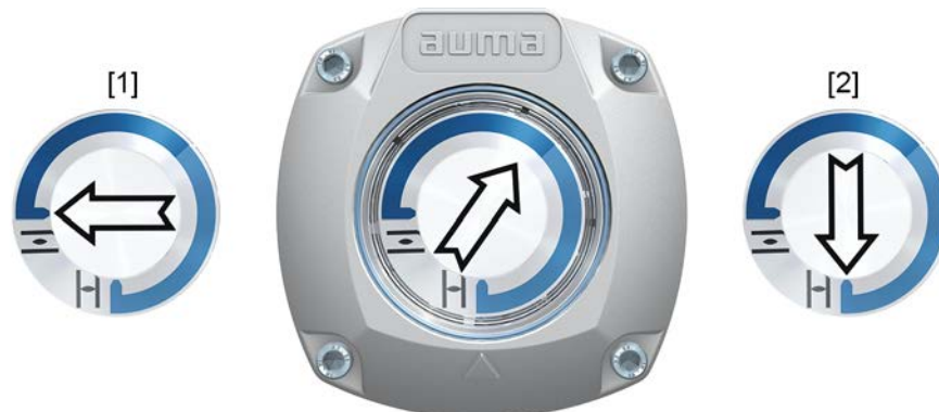
Figure 65: Mechanical position indicator
