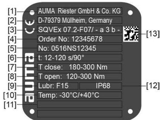
Figure 5: Actuator name plate (example)
