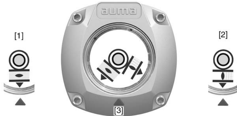
Figure 66: Mechanical position indicator
