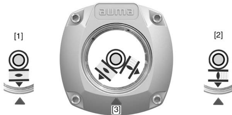
Figure 69: Mechanical position indicator
