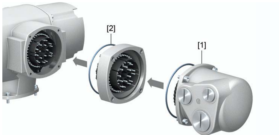
Figure 36: Electrical connection with DS intermediate frame
