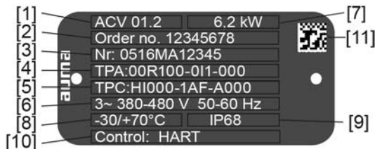
Figure 6: Name plate for actuator controls (example)
