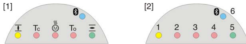
Figure 67: Arrangement and signification of indication lights
