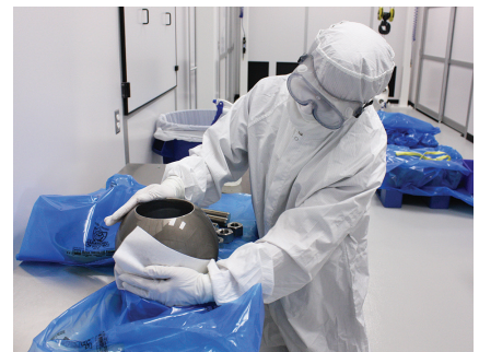
MOGAS' dedicated cleanroom prepares valves for an oxygen-enriched environment.
