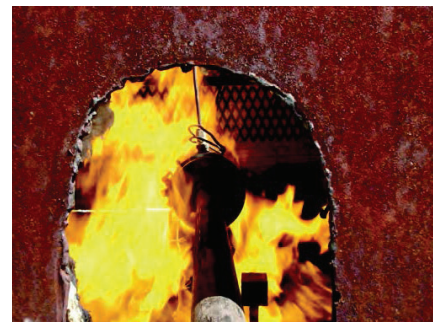
MOGAS Watson Series flanged ball valves are tested and certified to meet the fire test requirements of API 607.
