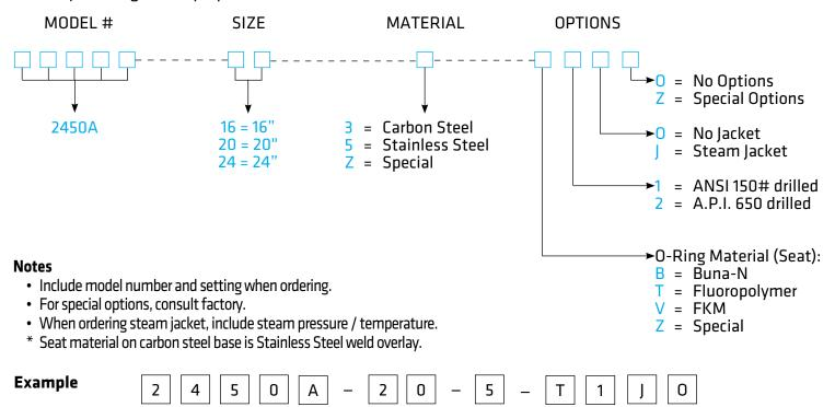
Indicates a 20" Model 2450A with Stainless Steel Body, Fluoropolymer Seat Diaphragm, ANSI 150# drilled, Steam Jacket and no other options.
