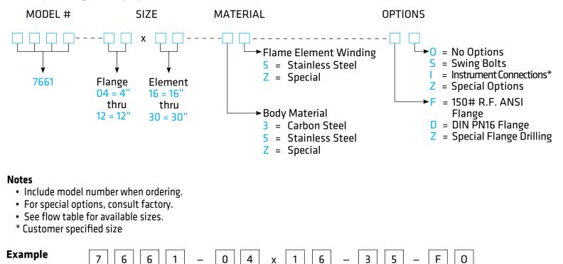
Indicates a 4" Model 7661 with Carbon Steel housing, 16" Stainless Steel Flame Element, ANSI Flanged Outlet and no other options.
