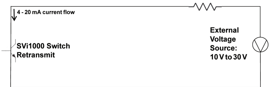
Figure 35 - Simplified Retransmit Option Installation Drawing
