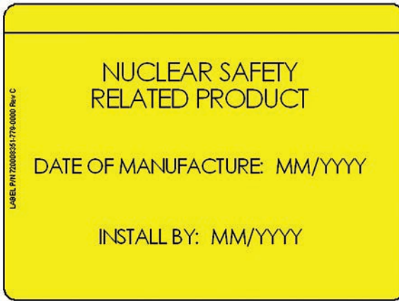
Figure 2 - Safety Related Nameplate
