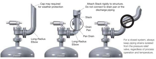
Figure 10: POSRV Parts Alignment
