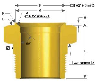
Figure 13: Nozzle O-Ring Seat (DA)
