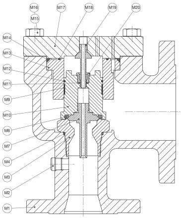
Figure 1: Main Valve Construction - Soft Seat
