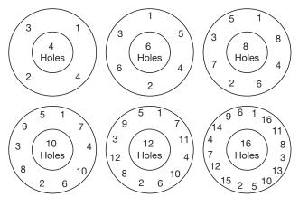
Figure 16: Bolt Tightening Patterns
