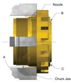
Figure 14: Machining Nozzle Seats
