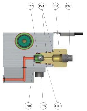
Figure 36: Field Test Connection Assembly
