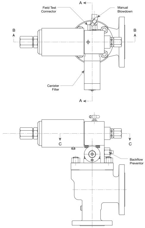
Figure 7: POSRV Assembly with MV22/72 Pilot
