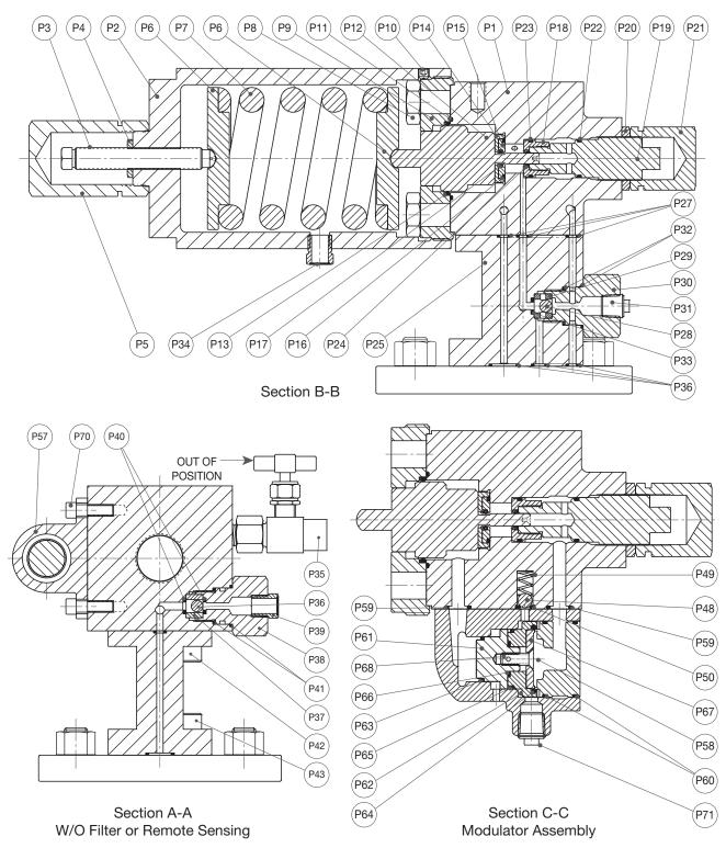
Figure 6: 49MV07 Pilot Valve Construction
