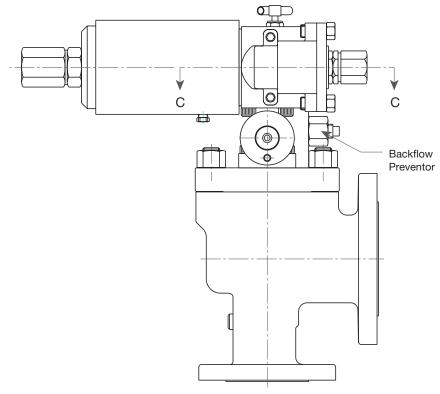
Figure 5: 4900 Series POSRV Assembly with 49MV07 Pilot
