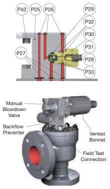
Figure 35: Backflow Preventer Assembly
