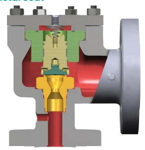
The Consolidated 3900/3900 TM Series POSRV is supplied with a non-flowing pilot valve. This single pilot design is well-suited for both incompressible and compressible applications and performs equally well on liquid, vapor or two-phase flow services. The set pressure will not require adjustment if service conditions change.
